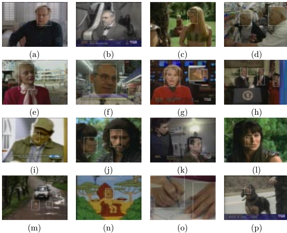
Figure 9: The boxes indicate the faces detected for C \leq 20 .
